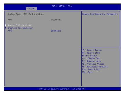
The Chipset menu controls the system's chipset.
