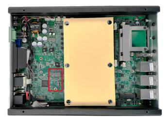
Prepare the Wi-Fi module kit. The module is a M.2 E-Key socket form 3. factor, with two MHF connectors, one is "MAIN", and the other is "AUX".
