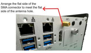
11. Mount the washer first and then the nut to the SMA connector. Make sure the nut is tightened.
