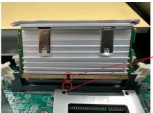
Align the notch on -the memory module with the notch in the memory socket.
