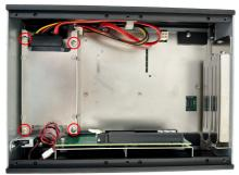
3. Slide the HDD/SSD storage device into the bracket and fix the storage device in place by fastening the 4 screws on the bracket.
