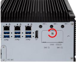
2. Position the CFast/SIM card as directed by the graphic printed on the front panel. Insert the CFast/SIM card all the way into the slot.
