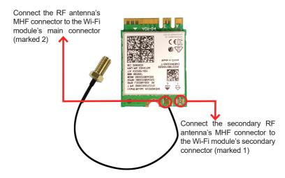
6. Plug the Wi-Fi module to the socket's connector by a slanted angle. Fully plug the module, and note the notch on the wireless module should meet the break of the connector.
