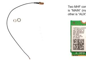
Two MHF connectors, one is "MAIN" (marked 2), the other is "AUX" (marked 1).
